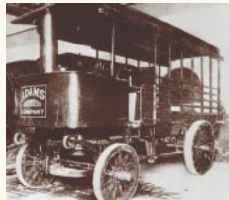
Powered by a heavy steam engine, this 1900 Adams Express wagon negotiated the cobblestone streets of Philadelphia on extra wide wagon tires.
